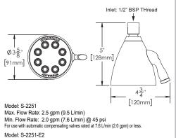
Model: S-Z251-E2 Max. Flow Rate: 2.0 gpm (7.6 L/min) Min. Flow Rate: 1.5 gpm (5.7 L/min) @ 45 psi For use with automatic compensating valves rated at 5.7 L/min (1.5 gpm) or less.
